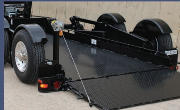
Crank down tailgate/ramp allows a minimum angle for low ground clearance equipment.
