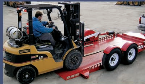
A flip of a switch hydraulically lowers the deck to ground height to allow fast, drive-on access.
